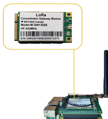
Fig. 4 LoRa Gateway (Raspberry Pi + SX1302)
