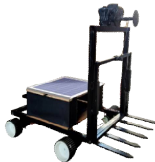
Fig.1. Actual image of project (Arduino-based Solar powered Mini Forklift)
