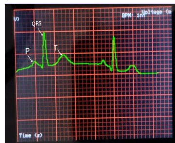
Fig. 11b PQRS Waveform Captured During Testing
