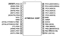
Because of its advanced RISC design, the ATmega328P is a high-performance, low-power 8-bit AVR microcontroller that can execute 131 strong instructions in a single clock cycle. It's a CPU that's typically seen in Arduino boards like the Arduino Fio and Arduino Uno.
