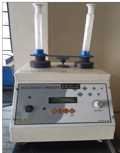
Fig. 2. Bulk Density Apparatus Measuring Bulk Density of Powder
