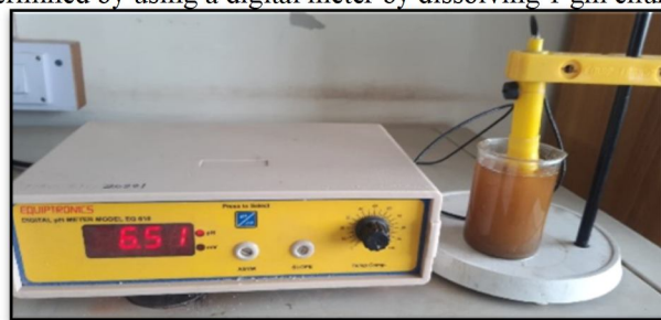
Fig. 1. Digital pH meter Measuring the pH of the Powder
