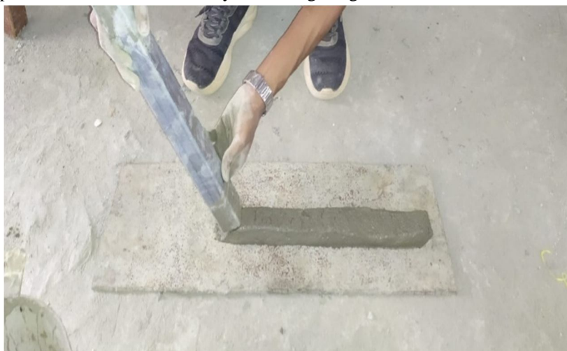
Figure 2: Prototype (GI pipe) used for extrudability testing
