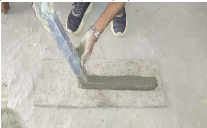
Figure 2: Prototype (GI pipe) used for extrudability testing
