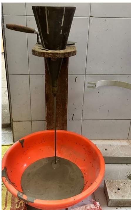
Figure 5: Marsh cone test assembly
