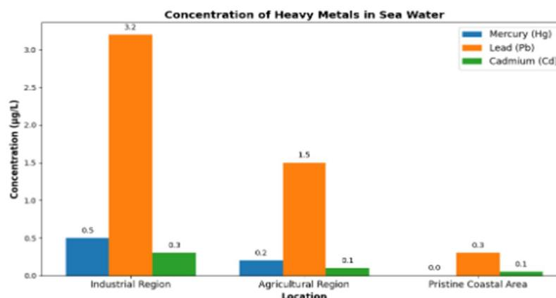
These results indicate a direct influence of industrial activities on the concentration of heavy metals in sea water. Elevated concentrations in the industrial region suggest contamination from industrial discharges and effluent contamination.
