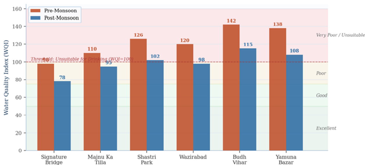
Figure 6: Water Quality Index — Pre-Monsoon vs. Post-Monsoon (2025). Coloured bands indicate WQI classification zones. Dashed red line at WQI = 100 marks the 'Unsuitable for Drinking' threshold.
