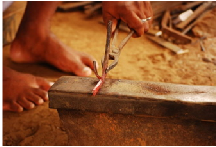
Fig.7 Bending Metal to Form a Shape
