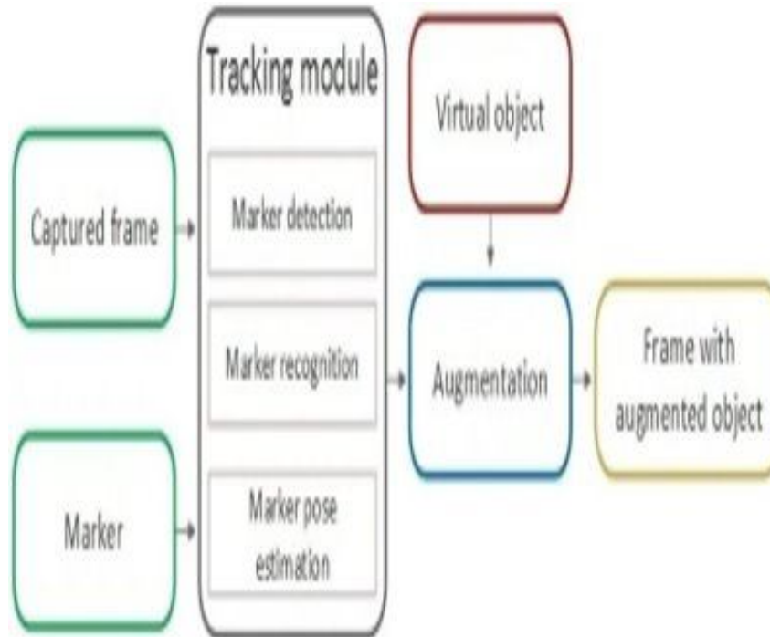
Fig. 3 Working Model of AR core
