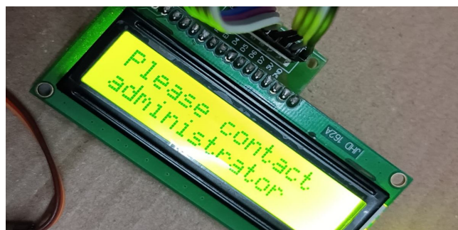
Fig. 16. LCD Output When an Unauthorized Vehicle Enters
