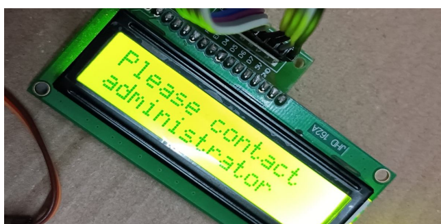
Fig. 16. LCD Output When an Unauthorized Vehicle Enters
