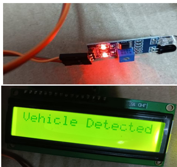
Fig. 2. IR sensor and LCD Output When a Vehicle is Detected Within Range.
