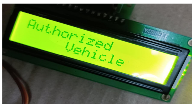
Fig. 13. LCD Output When an Authorized Vehicle Enters
