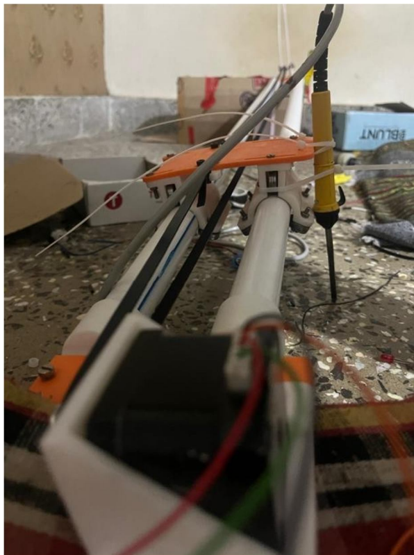
Fig3. Stepper Motor Connected with Conveyor Belt
