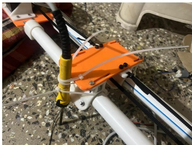
Fig4. display the soldering gun connected with the conveyor belt. stepper motor moves the soldering gun using conveyor belt
