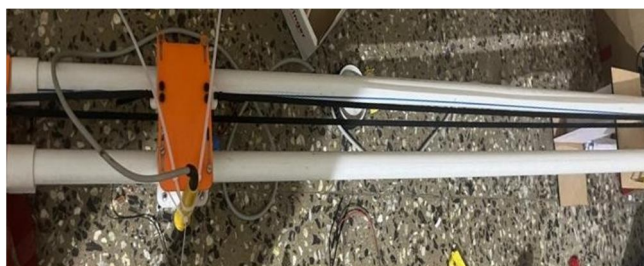
Fig5. Displays the main part of the system, the soldering gun move with conveyor belt while rotating the stepper motor. The soldering gun move with bearings for smooth movement
