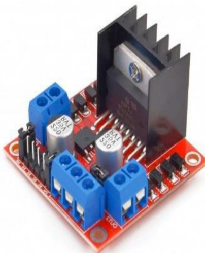
Figure 4 H-Bridge for Motor and Sensor power distribution
