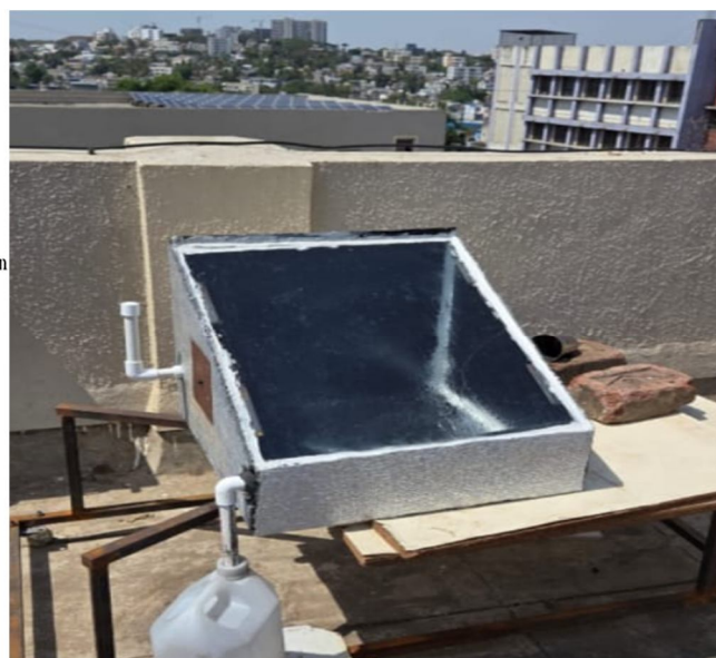
Figure 2: Prototype implementation of the dual-axis solar tracking and distillation system.
