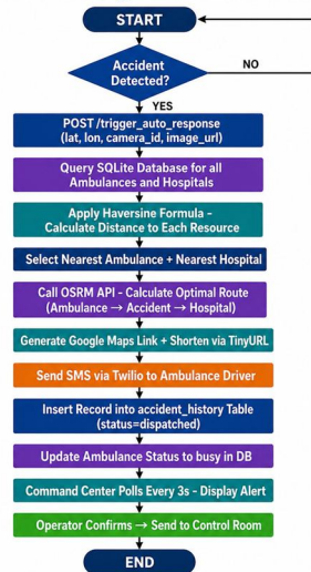
Fig. 4. The software design flow of AERS demonstrates its complete detection-to-dispatch process which begins with accident confirmation and continues through Haversine resource selection and OSRM routing and SMS dispatch and operator handoff to the Control Room.
