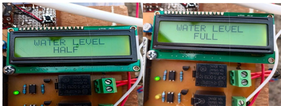
Figure 5: Displaying available Water level in container
