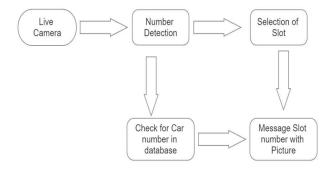
Once the numbers from the number plate are obtained, that number is checked from the database to obtain the owner's info, once we get that information a basic linear algorithm isrun to assign the nearest slot for the car, and the slot details along the map route is sent to the owner's message, which can be followed along to reach the allotted slot.
