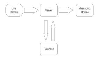
A camera near the society gates that can record images of automobiles together with their licence plates and send them to the server runs an algorithm to extract only the licence plates from the obtained picture. The number plates are retrieved using the clever Edge detectors, which will onlyidentify the automobile number plates in the image and delete all other unneeded elements.
