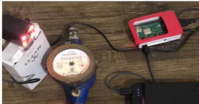
Fig. 5 Automated Water Meter Reading System
