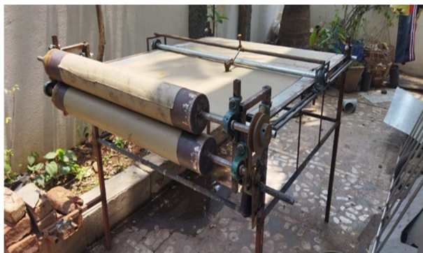
Fig.8. Main setup of automatic lamination cutting machine
