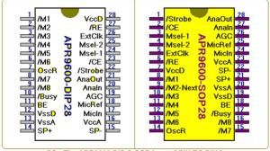
PS: The APR9600 DIP & SOP is not [ PIN TO PIN ]
