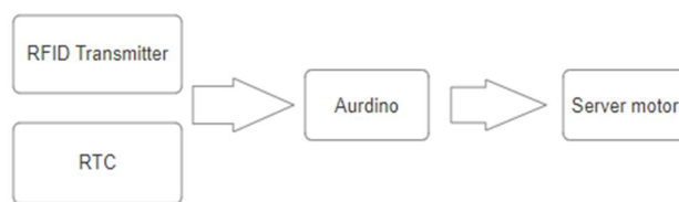
Fig.1 Block Diagram for automatic pet feeder
