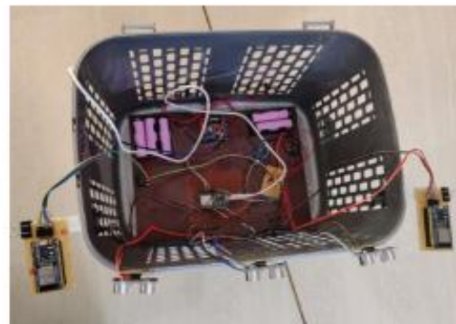
Fig.6 Final Prototype of the Autonomous BLE-Based Smart Shopping Trolley
