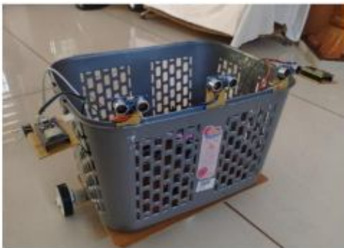
Fig.6 Final Prototype of the Autonomous BLE-Based Smart Shopping Trolley
