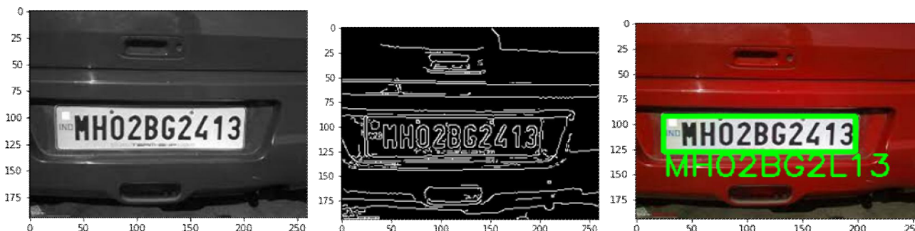
Figure 10- Limitation In Plate Recognition
