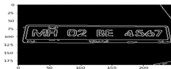
Figure 5 – Canny Edge Detection on Masked Image
