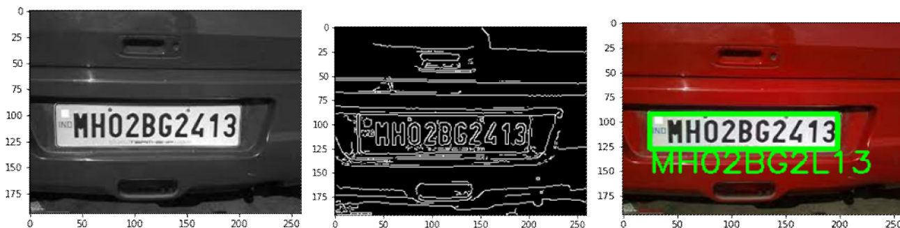
Figure 10- Limitation In Plate Recognition
