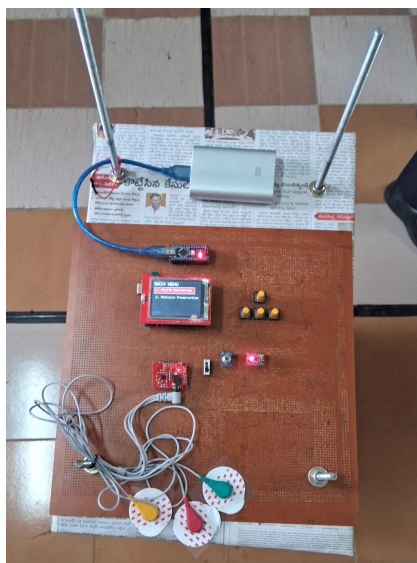
Fig no 13: Top view of robot depicting the health monitoring system
