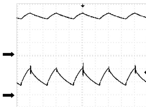
Figure 7 – LEDs lamp voltage (UP) and current (DOWN) (20V/div; 0,5A/div; 10μs/div).
