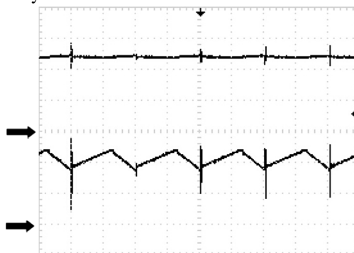
Figure 6 – Batteries voltage (UP) and current (DOWN) (10V/div; 1A/div; 10 \mu s/div).
