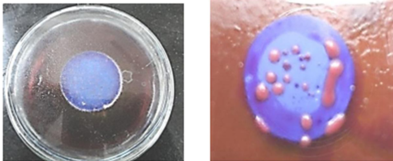
Figure 7: E. coli count by membrane filtration method
