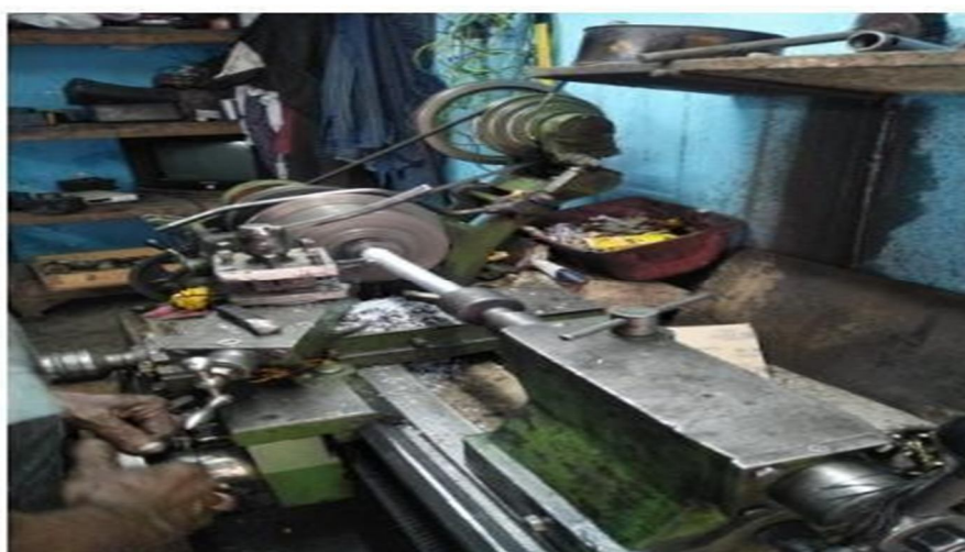
Fig: Turning process for Casting Component
