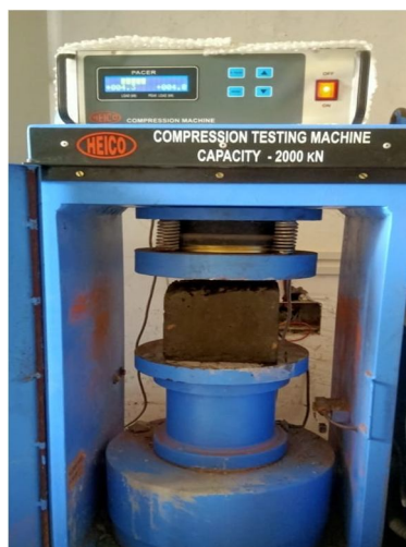
Figure 3.3.4: Concrete cube placed under Universal Testing Machine
