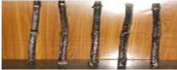
Figure.3.2: Bamboo sticks after treatment with coal tar.
