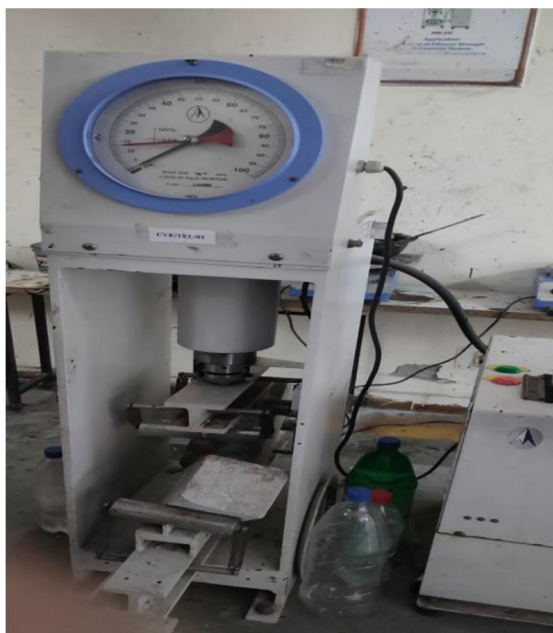
Fig. 4.8 Determining the flexural strength of the beam through ASTM
