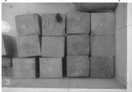
Fig.5.2.4 Curing of cubes
