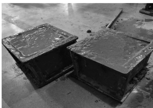
Fig.5.2.3 Casting of cubes
