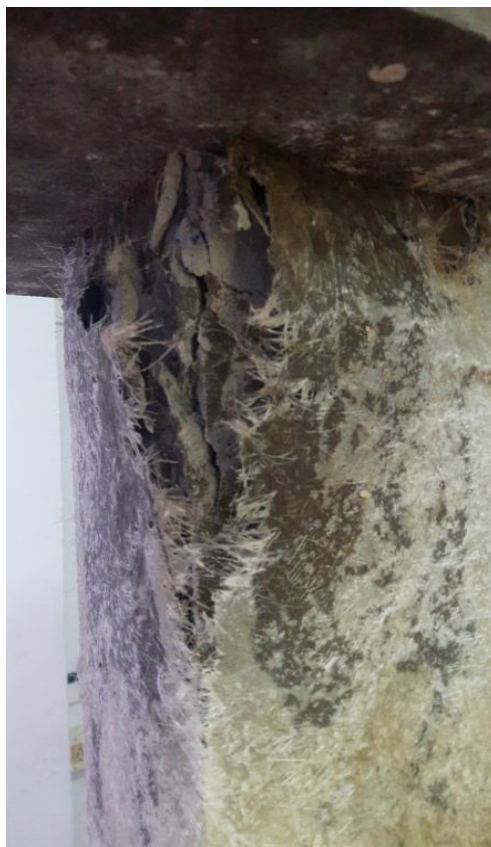
Fig. 14 Compressive Strength of Column Test
