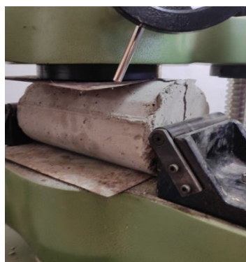
Fig. 12 Split Tensile Strength of Concrete Test
