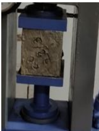
Fig. 10 Compressive Strength of Concrete Test
