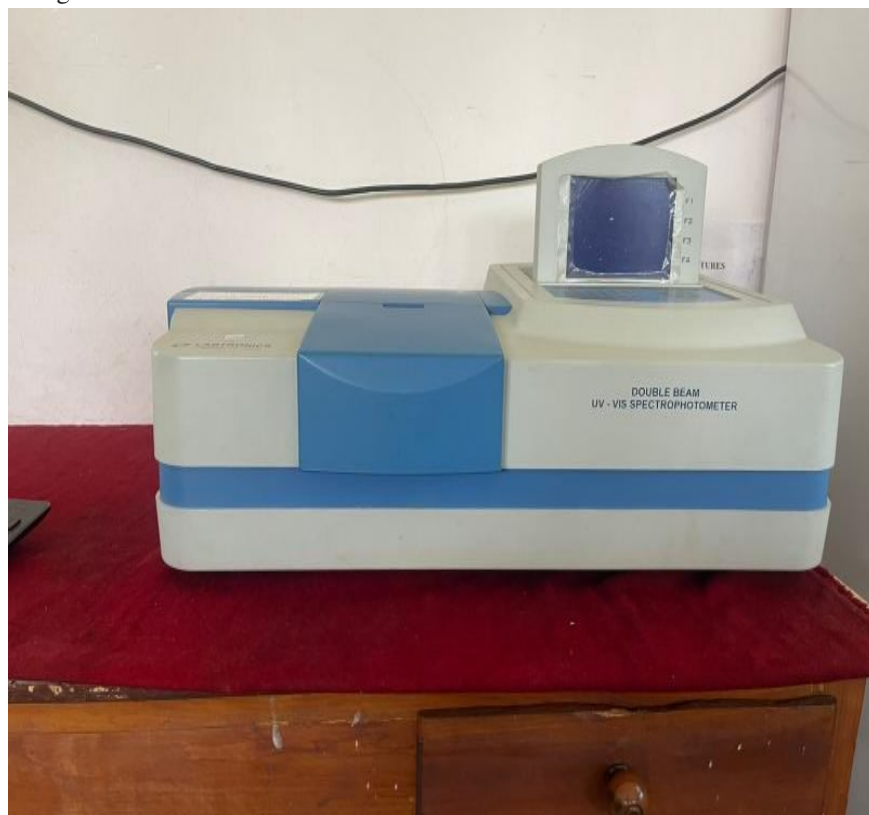
Figure 20: Double Beam UV -VS Spectrophotometer
