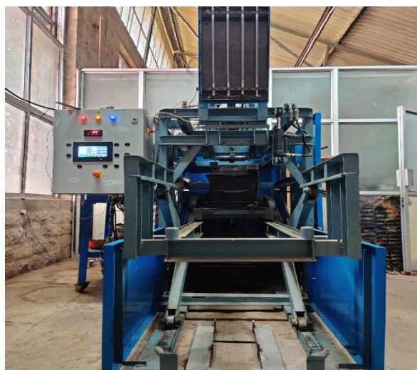
Fig. 1 Roller compactor and rut analyser
