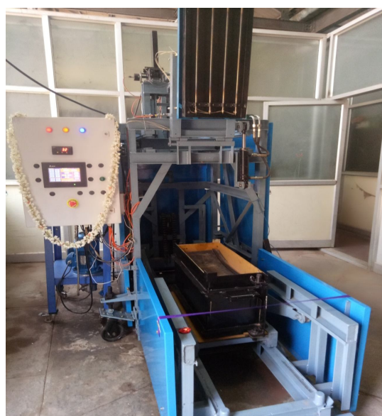
Fig: Roller Compactor cum Rut Analyzer (RCRA)
