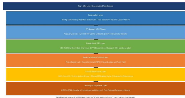
Fig. 1. Six-Layer Decentralized System Architecture
