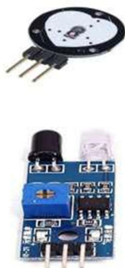
Fig1: Heart Rate Pulse Sensor Module & IR (Infrared) Sensor Module for Hemoglobin.
