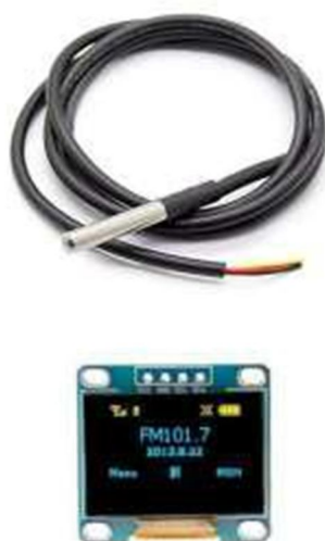
Fig 2: DS18B20 Water Proof Temperature Sensor Probe & Oled display.
