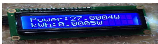
Fig-10.2 Power and kWh in LCD Display
