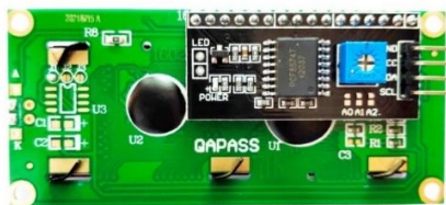
Fig-4 LCD with I2C Adaptor
