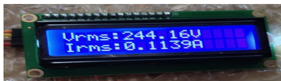
Fig-10.1 RMS value in LCD Display
