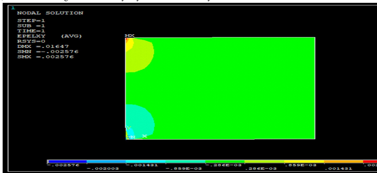
Figure 13: xy shear elastic strain for h/b .16 value and Carbon Composite Material
