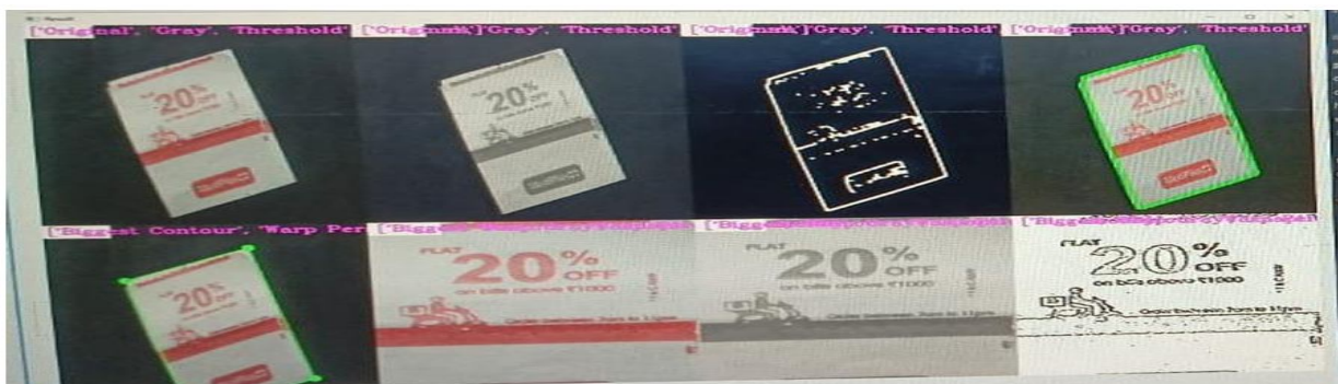
Fig. 1. Transformation of a Sample Document using various Image Processing and Computer Vision Techniques.
