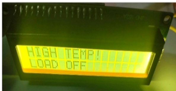
Fig. 4. LCD showing the “HIGH TEMP! / LOAD OFF” protection warning.
