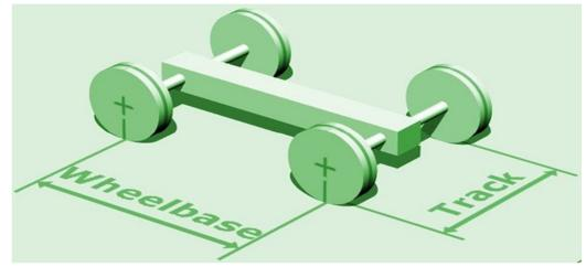
The dimensions of our solidworks design was determined on the basis of the length of the road/ track. The length of our track was \_\_\_\_\_ hence the TW of our vehicle is 120 cm. The WB in our vehicle is 68 cm, the WB is slightly shorter than the original WB, we decided to shorten the length to improve the movement of tires (In case of longer WB the tires were under a lot of friction which made the turning difficult).
