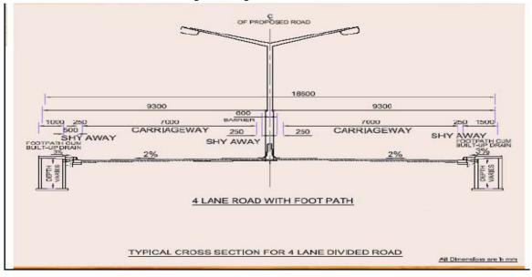
The following improvements are recommended: Road widening. Central median. Paving shoulders. Black topping metalled roads. Drains. Street lighting.
