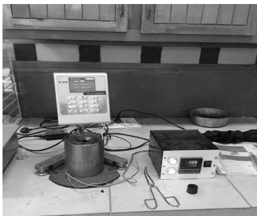
Fig. 3 EVALUATION OF VISCOSITY BY ROTATIONAL VISCOMETER
