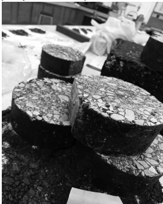
Fig. 4 NANO CLAY MODIFIED BITUMEN MOULDS
