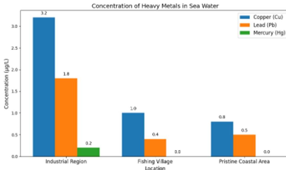
These elevated levels of copper and lead in the industrial region can be attributed to industrial runoff and sewage discharge, consistent with findings from Wang *et al.* (2015). Elevated mercury levels in coastal waters are often associated with industrial processes like mining and energy production, as described in previous studies.
