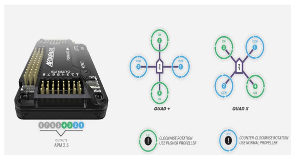
Fig 25 - Flight controller motor setup
