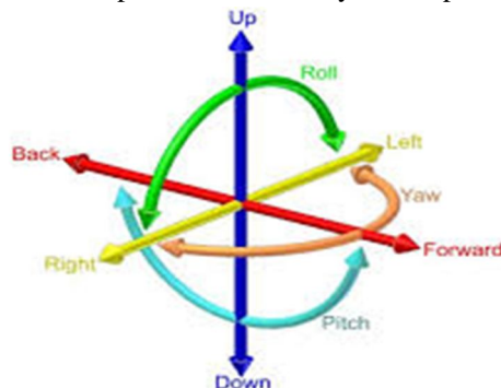
Fig 4 - Degrees of freedom in a quadcopter
