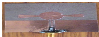
Figure 2 Fabricated CPW fed CMMA with radial stubs on magneto-dielectric substrate
