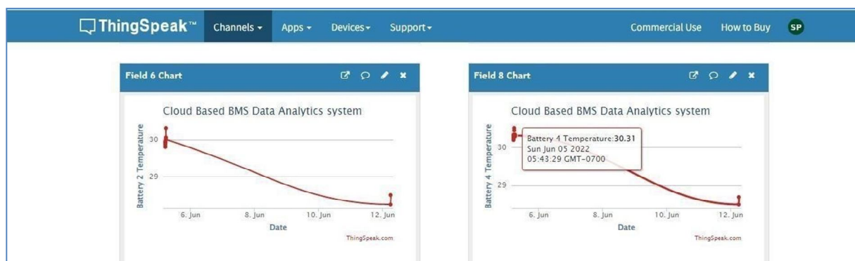
Figure 11: Graphical Representation of temperature of Lithium-ion cells
