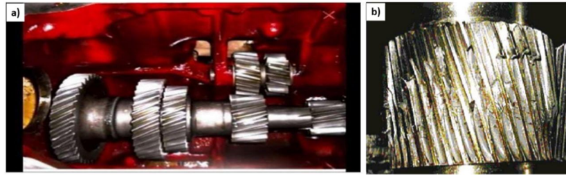
Figure 3: a) Gear box b) Damaged gear
